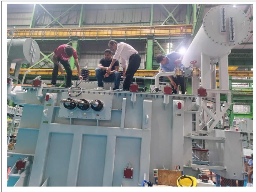
*Image 26: Transformer inspection at factory*
